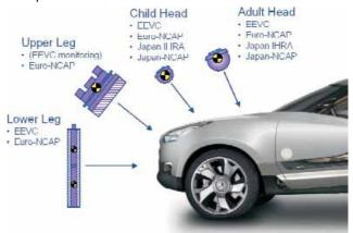
Figure 3. Graphical summary of the impact tests required under pedestrian protection legislation and consumer testing in Japan and Europe.
