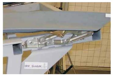
Figure 6b. Close-up detail of hinge attachment to support frame.
