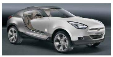
Figure 2: The Hyundai HED-4 QarmaQ advanced technology demonstration vehicle features a prototype hood made using IXIS thermoplastic composite technology.
