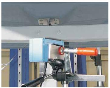
Figure 6c. Close-up detail showing the laser distancemeasurement apparatus positioned under the hood to measure intrusion into the engine bay.
