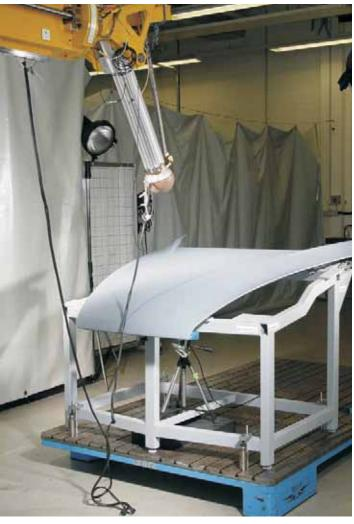
Figure 6a. Overall view of the impact testing set-up showing the hood assembly mounted on the support frame, impactor launcher and laser measurement device.
